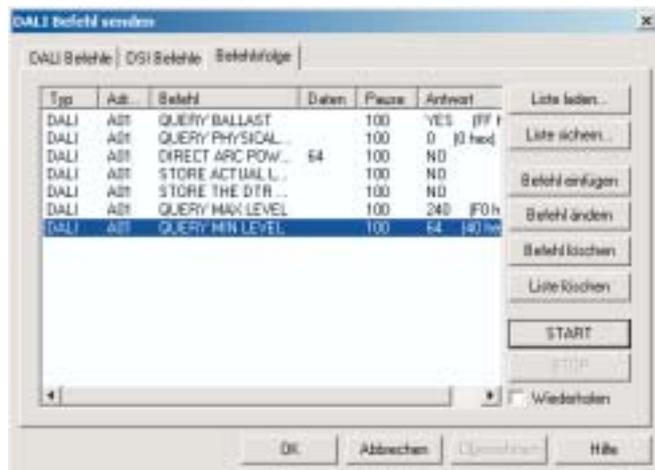
Use the tab "command list (Befehlsfolge)" to create and save command sequences, which will be used frequently. A command list may be helpful for initial initialization of the interface: set and store values for min level, max level etc.
